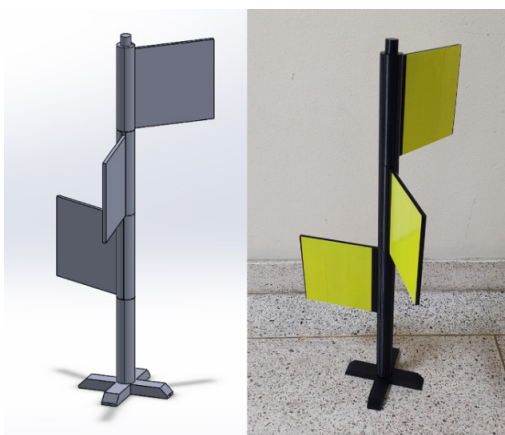
[Fig. 2] Model picture: Left picture - 3D modeling of the designed model for indoor experiment using solidworks. Right picture - model used for indoor experiment printed with 3D printer
