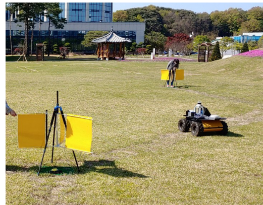
[Fig. 17] Outdoor Experiment: husky system running around the presented high intensity point generating model
