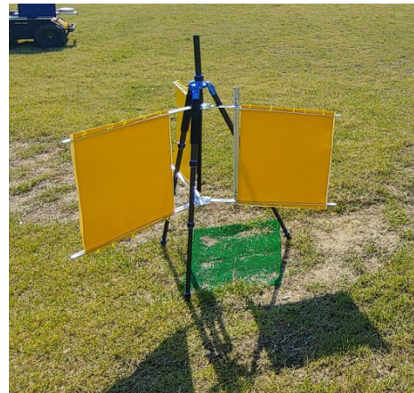
[Fig. 3] Model picture: Model used for outdoor experiment made with aluminum and high luminance sheet paper
