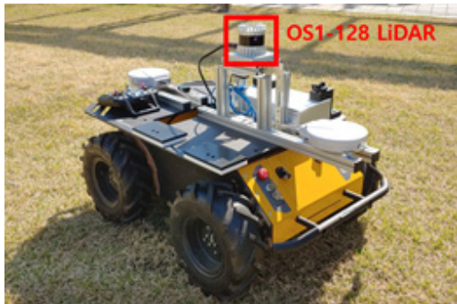
[Fig. 1] Husky Unmanned Ground Vehicle. Using Robot Operating System (ROS), it can move at a speed up to 1 m/s and climb a hill with an angular degree of 45°
